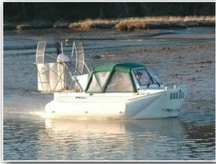
This latest update to the Vanguard series features a more powerful engine for increased speed, payload and headwind capability. The belt drive is designed to prevent any slippage, has improved efficiency, requires no re-tensioning, and eliminates the need for belt covers or touch bars, simplifying maintenance. The new idlers feature a double sealed bearing for greatly improved service life over the older v-belt idlers.
